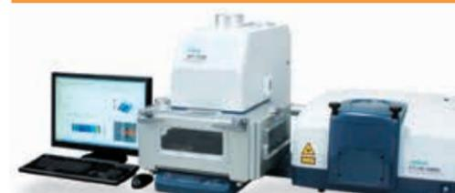
For FT-IR measurement, absorption peaks due to atmospheric water vapor and CO<sub>2</sub> can make it difficult to obtain high quality sample spectra. The most effective solution to this problem is the measurement of samples in vacuum. As a factory option, a vacuum type FT-IR microscope system can be provided.
