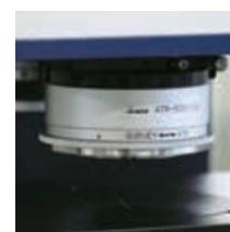
The "Clear-View" ATR objectives enable a simultaneous sample view even during ATR data collection after the ATR crystal element contacts the sample. The IQ Mapping function enables automated multi-point mapping, line mapping, grid mapping and IR Imaging analyses of a microscopic area with a manual sample stage and a single element detector.
