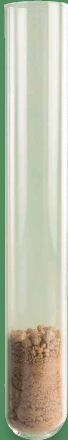
30 gram soil sample in disposable glass vials (actual size)
